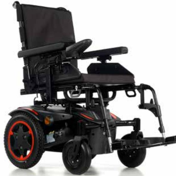
12.5" Drive wheels and 8" front castors provide a shorter base length for a tighter turning circle.
